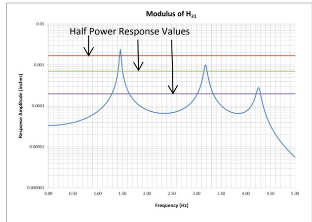
Figure 5 – Modulus Response of  $H(\omega)_{31}$
