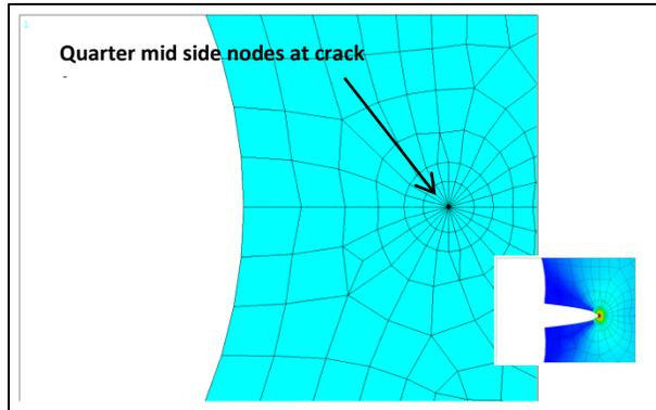
**Figure 3- Crack Front Mesh**
