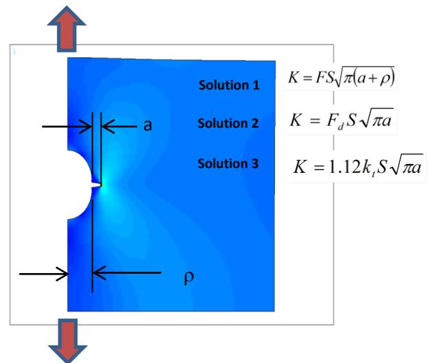
**Figure 1 – Half Model of Hole in Infinite Plate**
