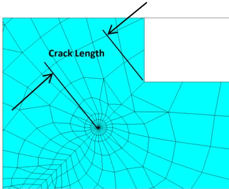
**Figure 11: Properly Aligned Crack Orientation**
