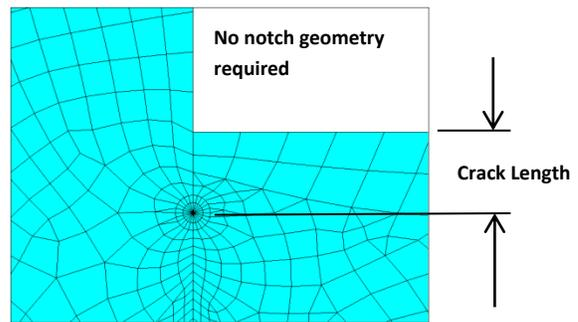
**Figure 10: Initial Crack Orientation**
