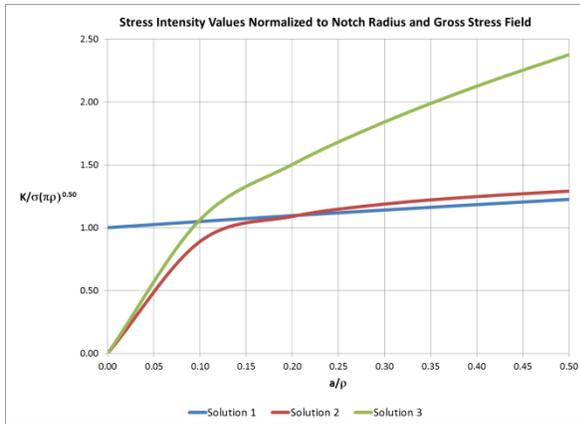
**Figure 2 – Normalized Stress Intensity Values**
