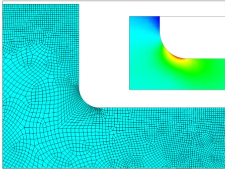
**Figure 7 – Mesh Density for Converged Solution**
